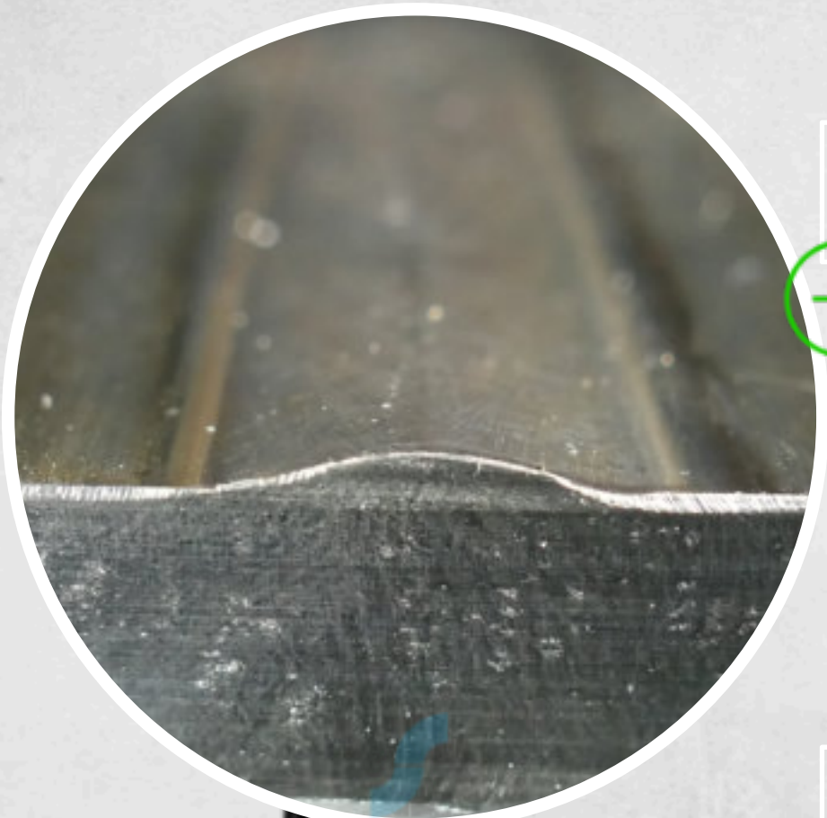
Stainless Steel Tank T: 10,0 mm Plasma Keyhole
