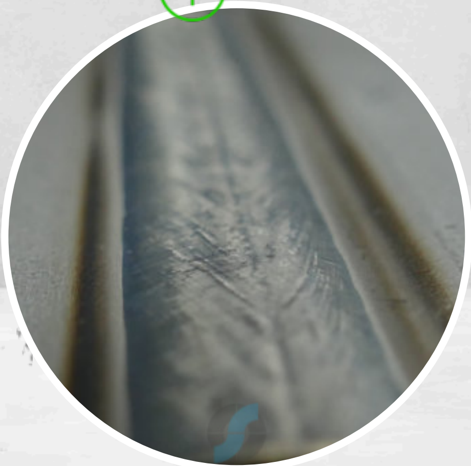
Stainless Steel vessel T: 6,0 mm High Performance TIG (inFocus)
