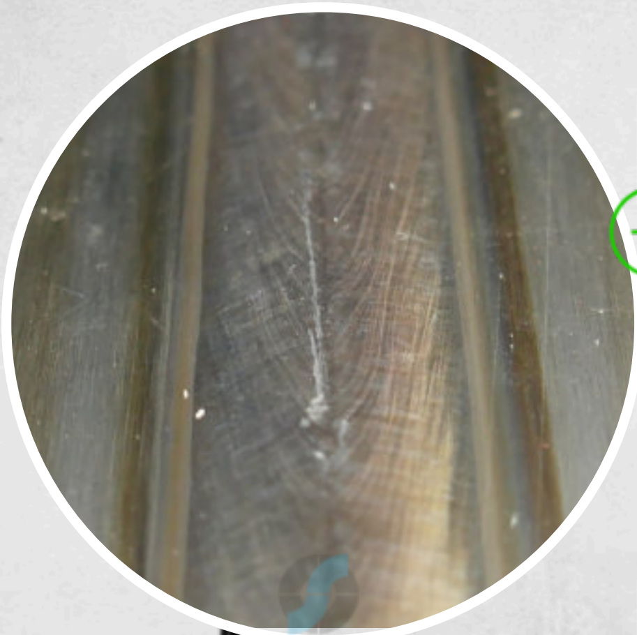
Stainless Steel Tank T: 10 mm Plasma Keyhole
