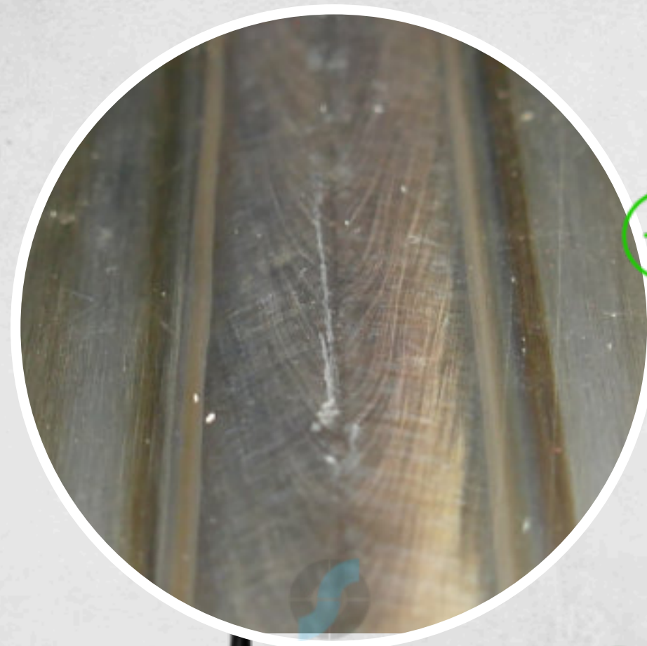
Stainless Steel Tank T: 10 mm Plasma Keyhole
