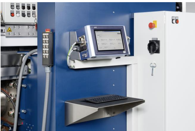
Figure 22: HKS Welding data monitoring system
