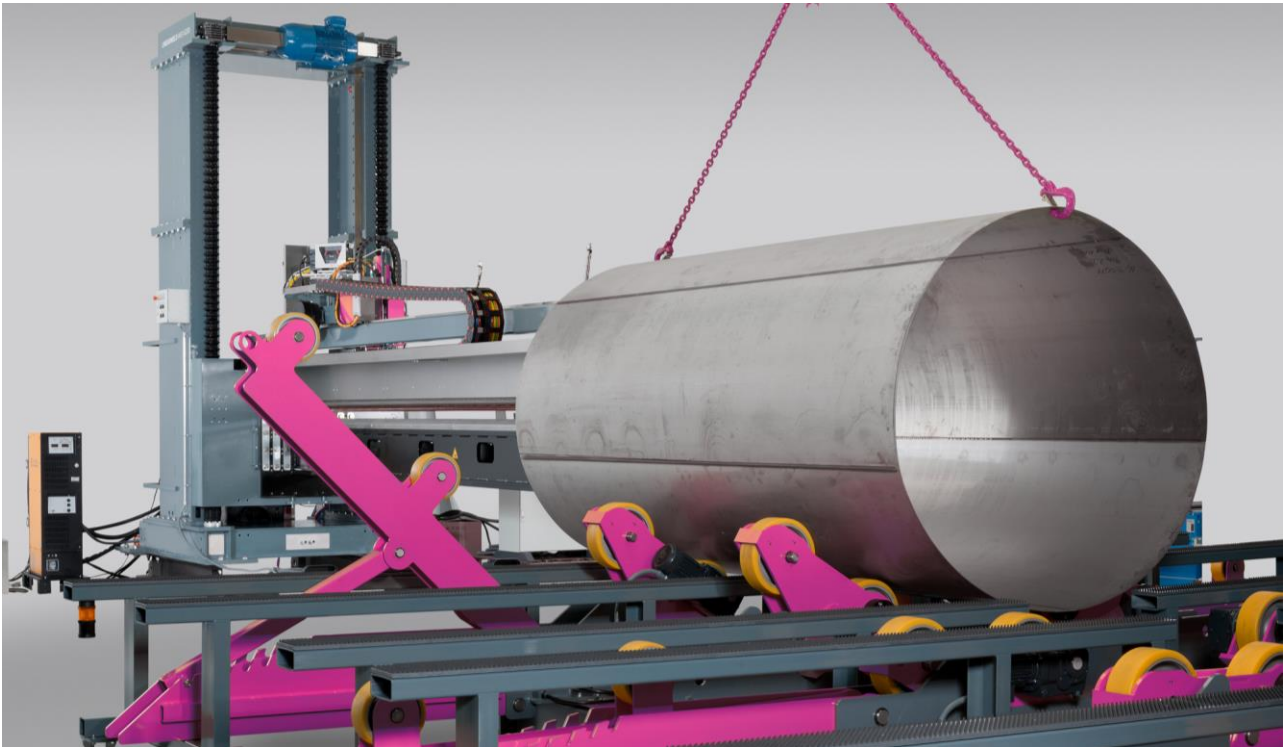
Figure 27 Insertion fit up truck with LINEARWELD INEX 6200
