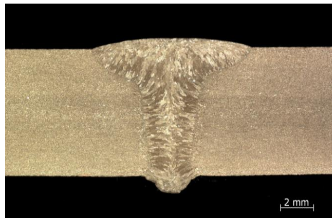
Figure 31: Plasma-Keyhole micrograph, t = 8 mm
