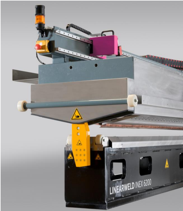
Figure 2: Mandrel latch, pneumatic actuated
