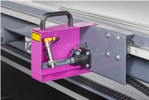
Figure 18: Centre mark with laser pointer
