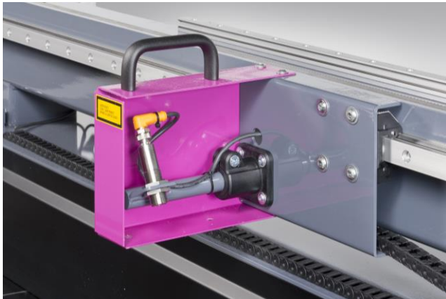
Figure 19: Centre mark with laser pointer
