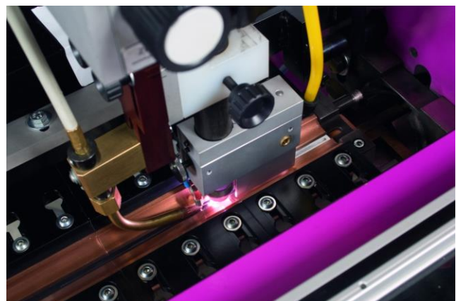
Figure 18: Coldwire unit with wire guidance
