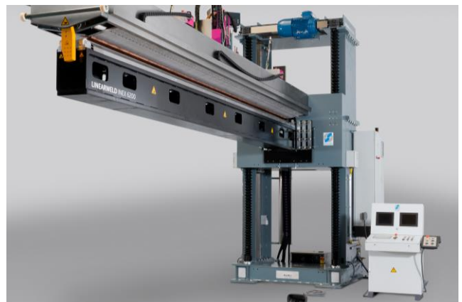
Figure 22: Electrical height adjustment, top position
