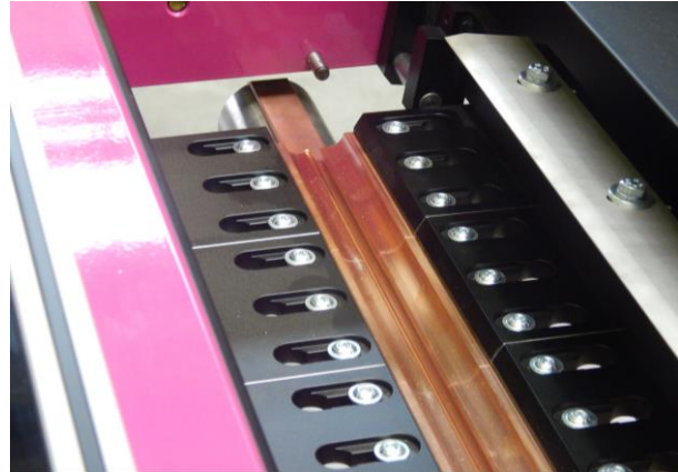
Figure 3: Clamping system with adjustable fingers
