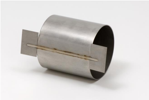
Figure 26: Stainless steel pipe t = 2,0 mm, TIG
