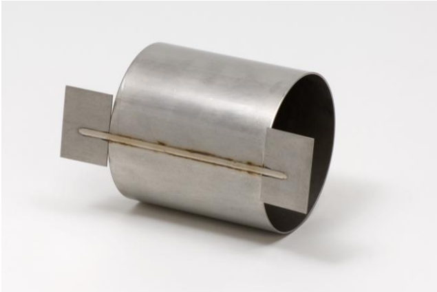
Abb. 26: Edelstahl Rohr t = 2,0 mm, WIG
