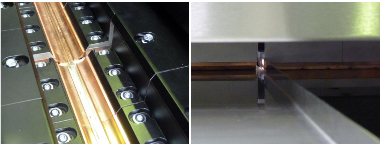
Figure 7: Outside clamping fingers with adjustable gap to accommodate mounting flange of box.
