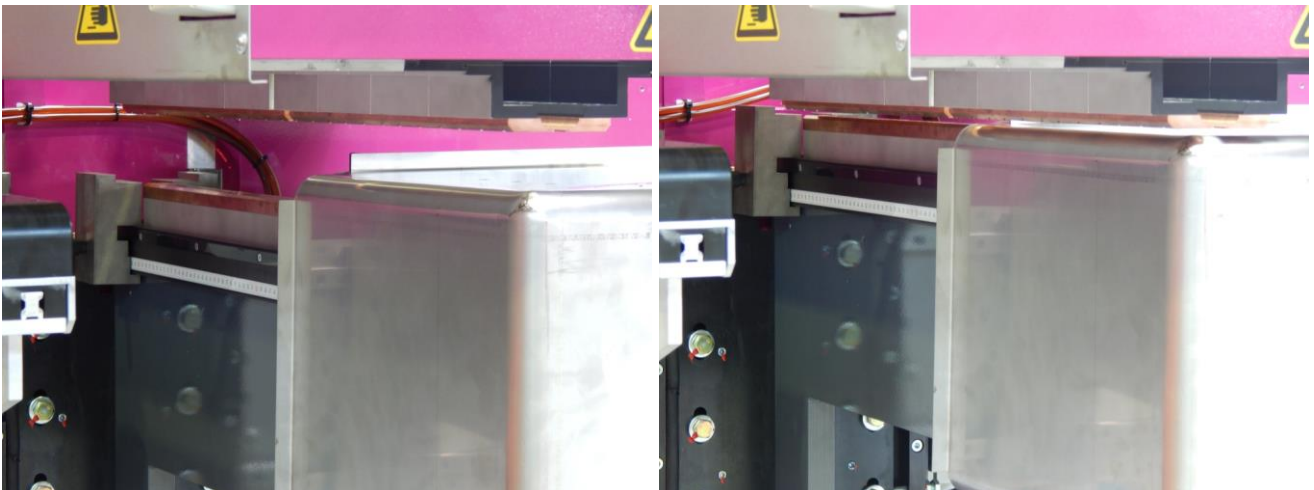
Figure 5: Mandrel Lift System for easy loading and un-loading, accommodates mounting flange.
