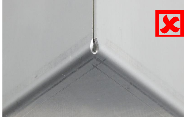
Abbildung 23: Biegeauge 1.4301 t = 1,0 mm
