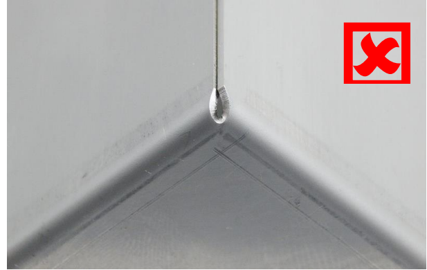
Figure 23: Bending eye 304 t = 1.0 mm
