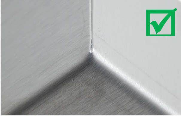
Figure 22: Bending eye 304 t = 1.0 mm
