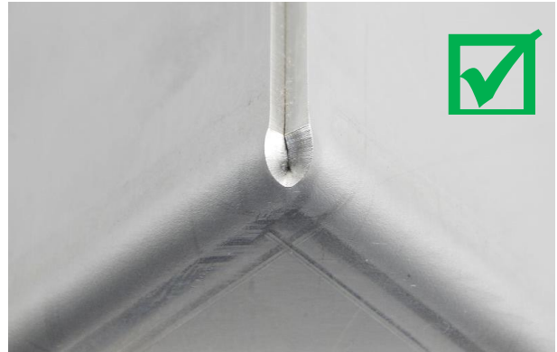
Figure 25: Bending eye 304 t = 2.5 mm
