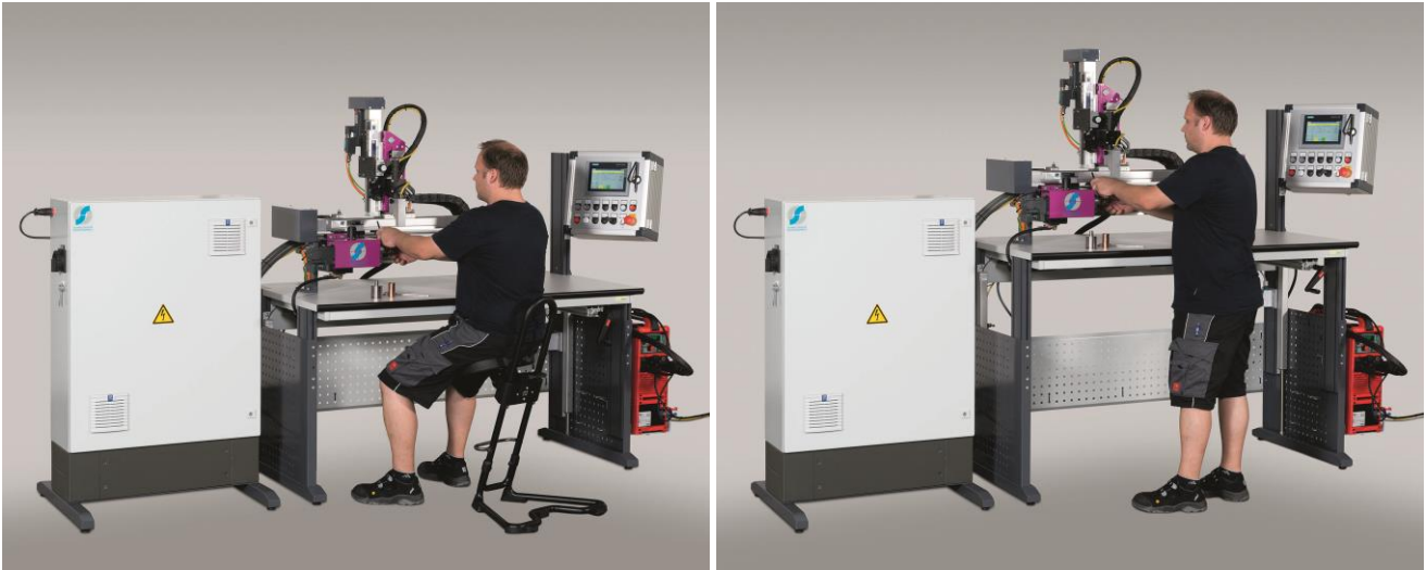
Figure 8: Ergonomic operation through height adjustable laboratory table (optional)
