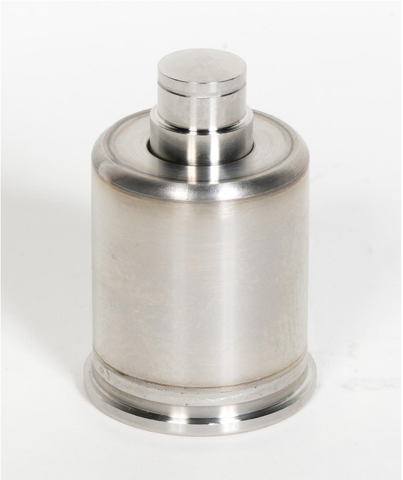
Figure 12: Welded part with 2 circumferential seams, as welded, \varnothing 40 mm, high alloyed steel
