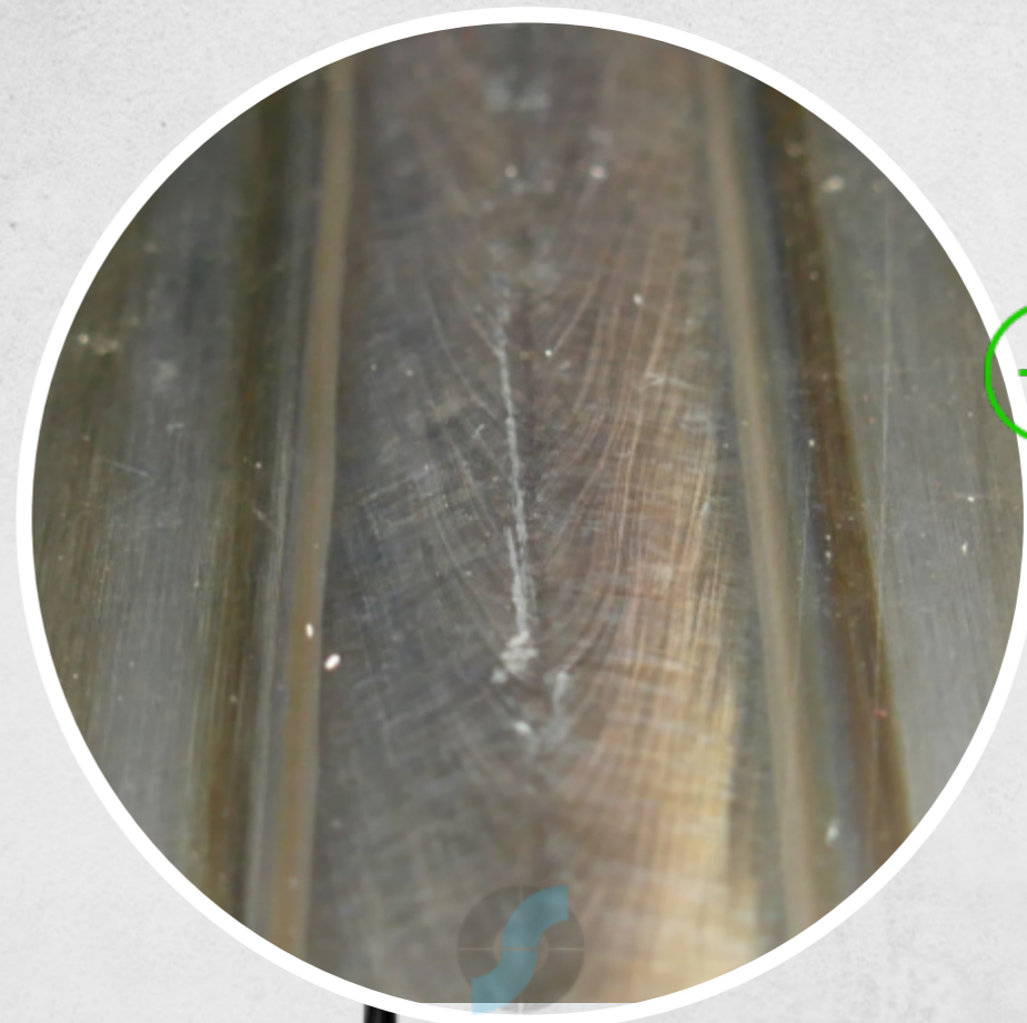
Stainless Steel Tank T: 10 mm Plasma Keyhole
