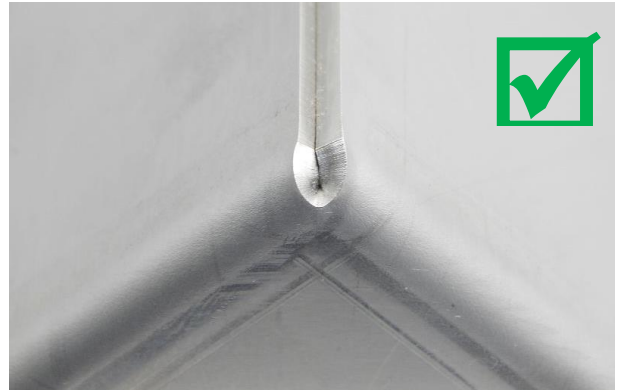
Figure 14: Bending eye 304 t = 2.5 mm
