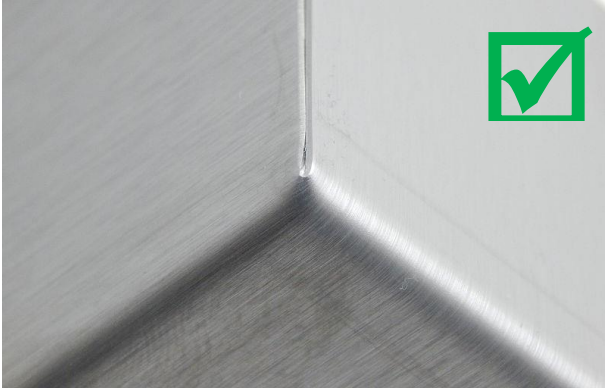
Figure 11: Bending eye 304 t = 1.0 mm
