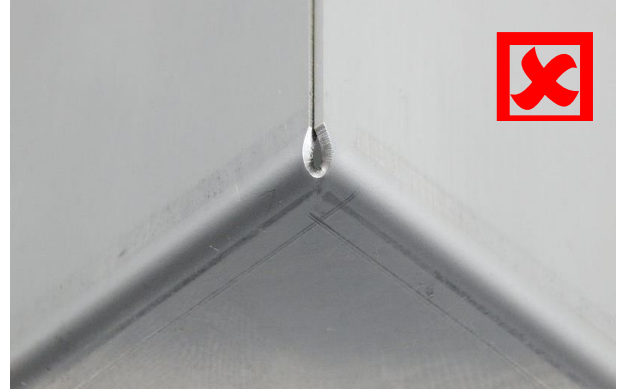
Figure 12: Bending eye 304 t = 1.0 mm
