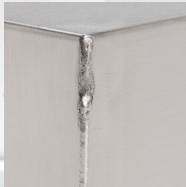
Manual welding and reworking
